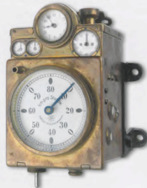
Geschwindigkeitsmesser Dr. Oskar Junghans, 1905 Dr. Oskar Junghans speed measuring device, 1905
