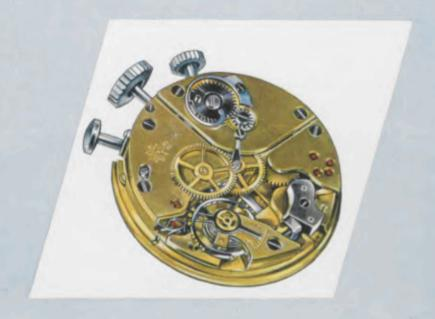
Solid lever movement J 89, with alarm, 20 jewels, shockproof. Nivarox hairspring, steel pallet and lever escape wheel, sweep seconds hand
