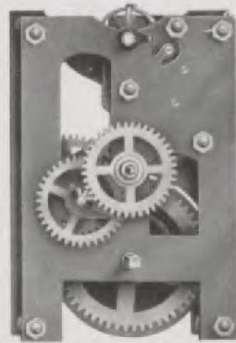
Platinen - plates - platines 6 x 9 cm = 2 1/4 x 3 1/2 inches
